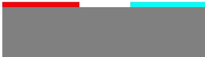
Figure 6.6: Considered planar device geometry. Grey denotes the semiconductor, while red and cyan denote the positive and negative electrodes, respectively. The semiconductor has a thickness equal to the length of the inter-electrode gap d and a width equal to 4d . The electrodes have an equal thickness of d/10 .
