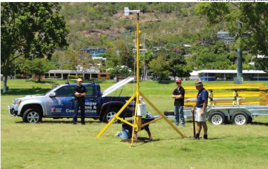
CTS staff with a portable anemometer used to measure wind speeds.
