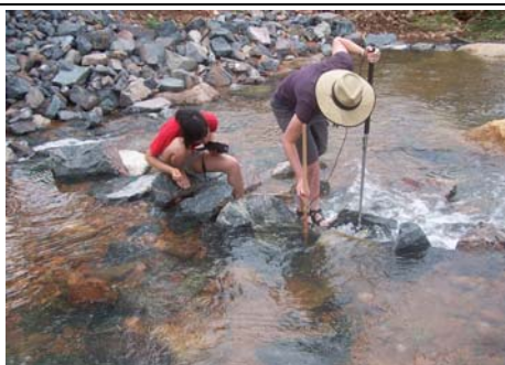
Velocity and flow depth measurements at rock ramp cascade # 2 (29/01/06)
