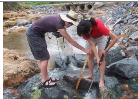
Velocity and flow depth measurements at rock ramp cascade # 3 (29/01/06)
