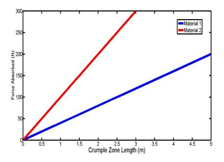
This graph shows how a crumple zone made of two different materials behave. Material 1 costs \$10 per metre, while material 2 costs \$30 per metre.
