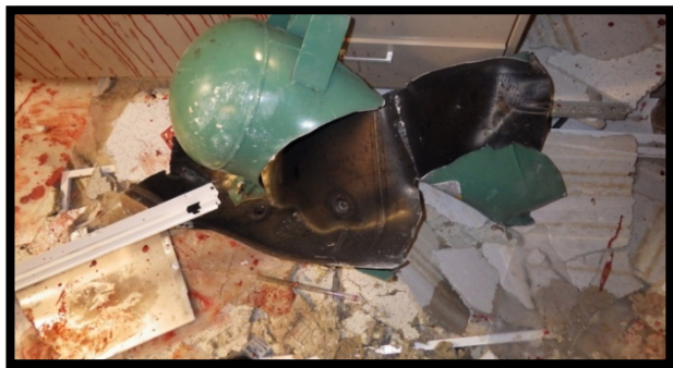
This steel tank ruptured during the explosion, which severed the researcher's arm.
