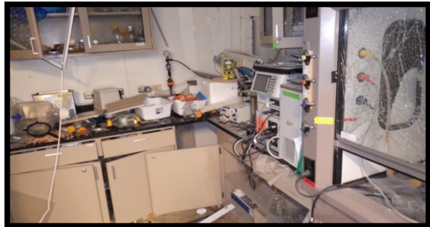
The explosion shattered fume hood windows and knocked over equipment.
