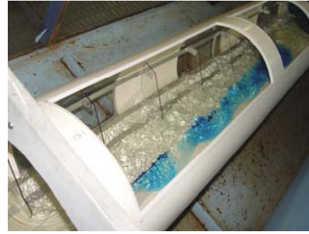
One standard baffle height flow depth: Dye inserted on right showing unobstructed flow outside baffle field on right (18/08/06)
