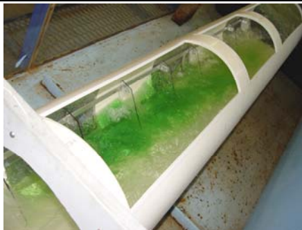
Two standard baffle height flow depth: Dye inserted in middle showing flow obstruction / shelter within baffle field on left (18/08/06)
