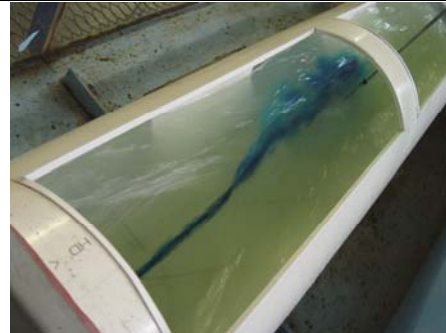
Three standard baffle height flow depth: Dye inserted in middle showing unobstructed central streamline above baffle field (18/08/06)
