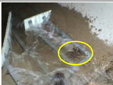
Glass perch moving through offset baffle fishway – schooling at downstream end within prototype fishway support cradle (28/01/06)
