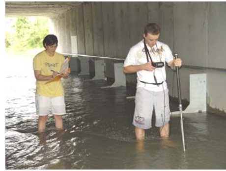
Velocity and flow depth measurements in culvert barrel #3 (11/04/06)
