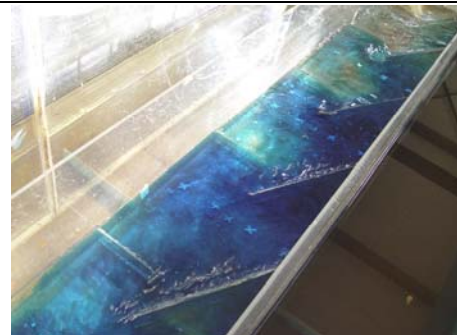
One standard baffle height flow depth: Time step 2; dye pattern showing shelter / flow retardance within baffle field (06/06/06)
